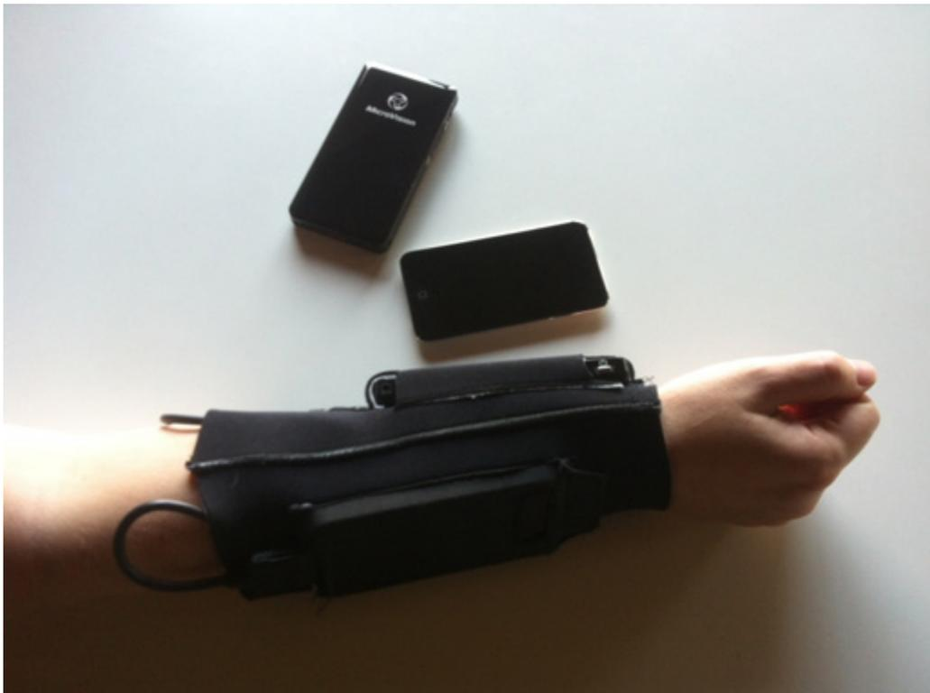
Figure 6 - S.A.R.A. – devices and neoprene arm sleeve
